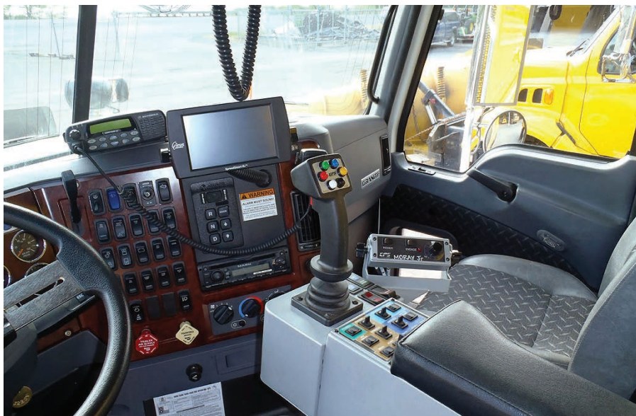
An ITD snowplow truck equipped with the SpreadSmart Rx electronic spreader control system from Certified Power Solutions.
