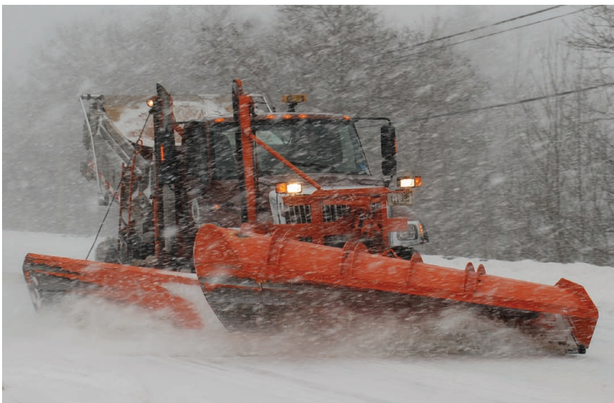
MaineDOT has outfitted its snowplow trucks with an electronic spreader control system that accurately records the amount of granular materials and liquids applied to winter roadways.
